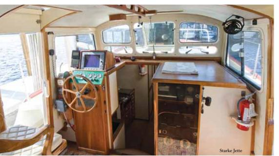
Opening ports forward, a sliding glass to port and starboard, and sliding hatches above the doors make for a well-ventilated deckhouse.
